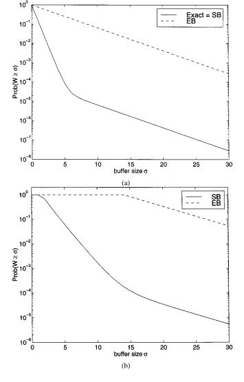
Fig. 2. (a) Bounding a distribution (exact) with a single exponential (EB) and with a sum of two exponentials (SB). (b) Bounds on the workload distribution of a multiplexer fed by two dependent processes: EB bound versus SB bound.
