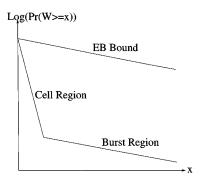
Fig. 1. Cell/burst regions, typical delay curve distribution, and EB bound.
