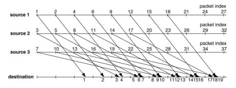
Fig. 7. Packet assignment to three sources and arrival times.
