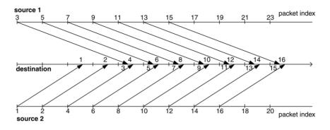
Fig. 6. Packet assignment to sources and arrival times.
