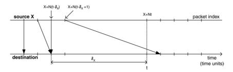
Fig. 4.  $\delta_X$  and the corresponding lowest indexed packet transmitted by source X that did not arrive at the destinations' receiver.
