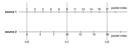
Fig. 5. Packet assignment for a = 5 and b = 3.
