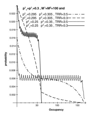
Fig. 11. Buffer occupancy probability-two sources with different transmission rates.
