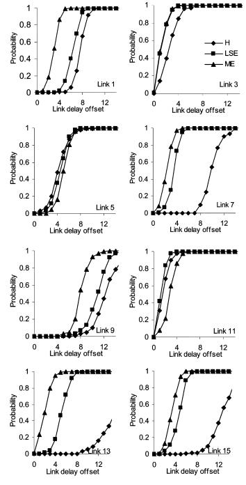
Fig. 4. The fraction of runs that the difference between the estimated link delay and the real link delay is not greater than t, for selected links in the fivr-node 16-links network.
