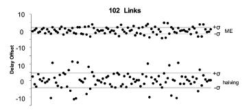
Fig. 10. The difference between the measured minimum delay and the estimated minimum delay. The standard deviation  $\sigma$  equals 1.9 and 4.4 for the ME and halving schemes, respectively.
