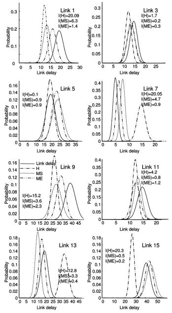
Fig. 5. Estimation of the normal distribution propagation delay in the five-node 16-link network. H—halving, MS—least square error, ME— maximum entropy.
