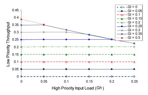
Fig. 9. Low priority throughput in a  $64 \times 64$  dual priority system under dual priority traffic. Gl represents the low priority input load.
