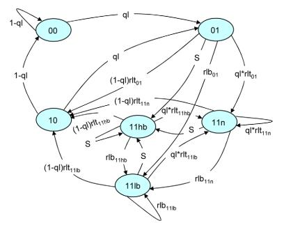
Fig. 15. The state transition diagram of a low priority queue in an SE(k) buffer.
