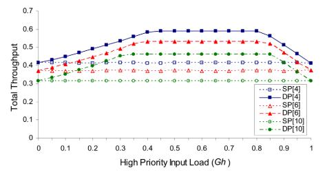
Fig. 6. Maximum total throughput of both single and dual priority systems under dual priority traffic (G = Gh + Gl = 1) as a function of the high priority input load (Gh) for various MIN sizes. SP[K] represents a single priority system with K stages MIN. Similarly, DP[K] represents a dual priority system with K stages MIN.
