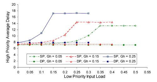
Fig. 11. Average high priority total delay in  $64 \times 64$  single priority (SP) and dual priority (DP) systems under dual priority traffic. *Gh* represents the high priority input load.
