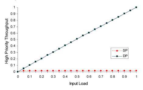
Fig. 5. High priority throughput in both single and dual priority systems with 6 stages under hot spot traffic. SP represents the high priority throughput in the single priority system, while DP represents the high priority throughput in the dual priority system.
