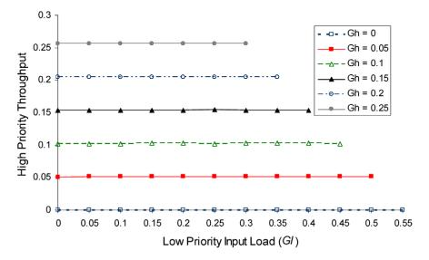
Fig. 10. High priority throughput in a  $64 \times 64$  single priority system under dual priority traffic. Gh represents the high priority input load.
