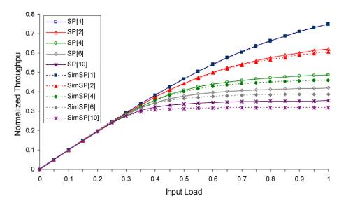
Fig. 14. Normalized throughput of a single buffered single priority delta–2 network for various network sizes. S[K] is the analyzed throughput for a network with K stages. Sim S[K] is the simulated throughput for a network with K stages.
