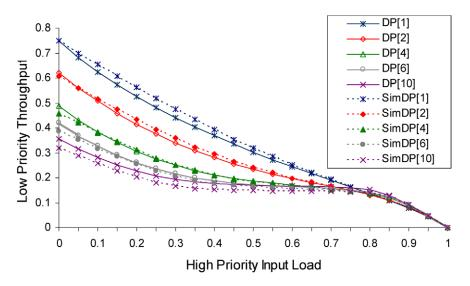
Fig. 16. Low priority normalized throughput of a single buffered dual priority delta–2 network for various network sizes as a function of the high priority input load, G. Sl[K] is the analyzed low priority throughput for a network with K stages. Sim Sl[K] is the simulated low priority throughput for a network with K stages. Low priority input load equals to 1–high priority input load.
