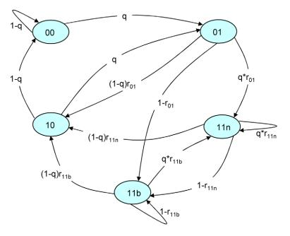
Fig. 12. The state transition diagram of a single priority SE(k) buffer.
