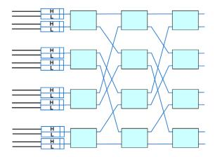
Fig. 4. An  $8 \times 8$  system: delta-2 network with input FIFOs.
