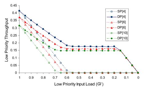
Fig. 7. Low priority throughput of both single and dual priority systems under dual priority traffic (G = Gh + Gl = 1) as a function of the low priority input load (Gl) for various MIN sizes. SP[K] represents the low priority throughput in a single priority system with K stages MIN. Similarly, DP[K] represents low priority throughput in a dual priority system with K stages MIN.
