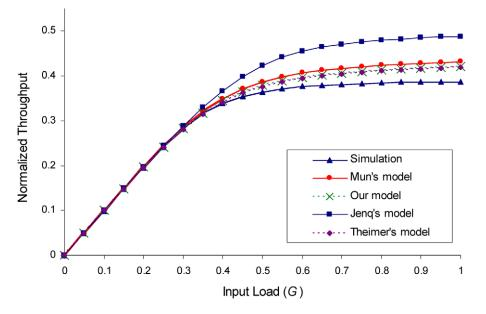
Fig. 13. Normalized throughput of a single buffered single priority delta-2 network with 6 stages.
