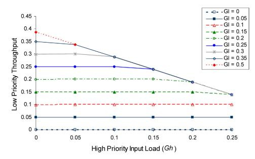
Fig. 8. Low priority throughput in a 64 × 64 single priority system under dual priority traffic. Gl represents the low priority input load.
